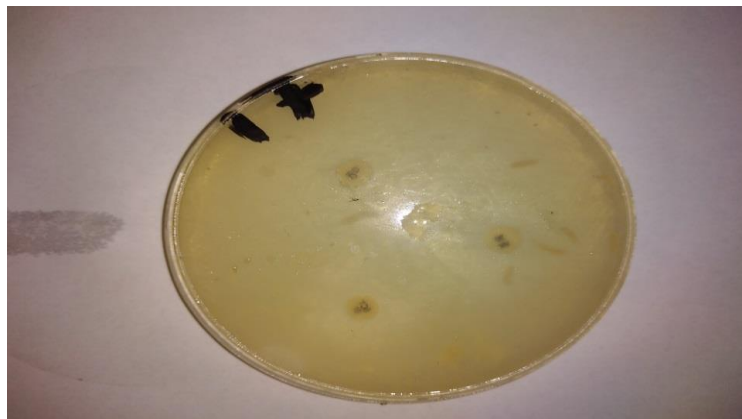
Figure 8: Antimicrobials susceptibility using Kirby bauer disc diffusion method
